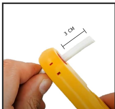
Remove 3cm cable jacket
